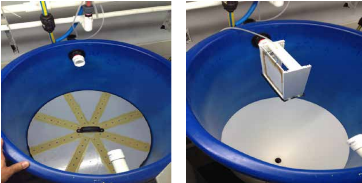
Figure 5. 270 Lt tank containing the false bottom (left) box filter with interchangeable screens (right).
