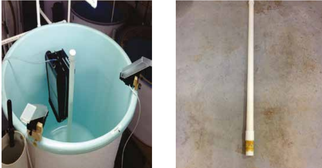
Figure 8. 1000 Lt tank and the locality of the filter, standpipe and feeders (left) 40 mm standpipe profile and the locality of the 10 mm holes (right).
