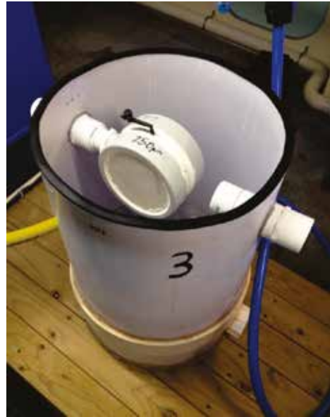
Figure 2. Banjo screen profile (left) and its locality in the 40 L tank, green arrow indicating poly valve and riser (right).
