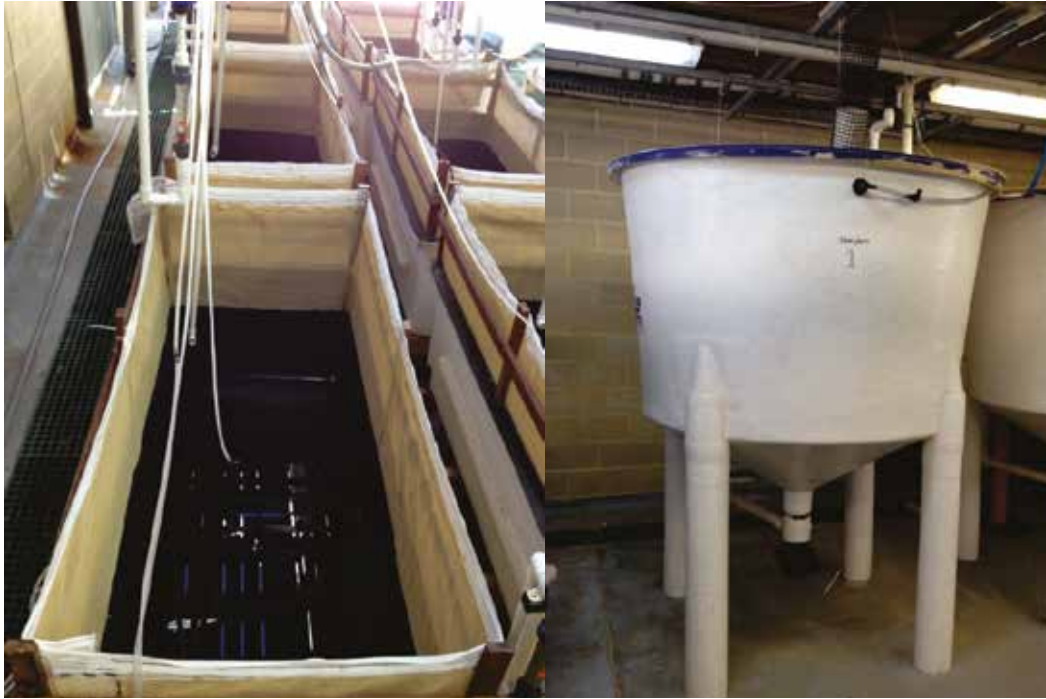
Figure 86 340L coffin tank used to house the female octopus tanks with eggs (left). 2000L tanks used for the high density grow-out trials and also for separating the octopus upon arrival to WAFMRL (right).
