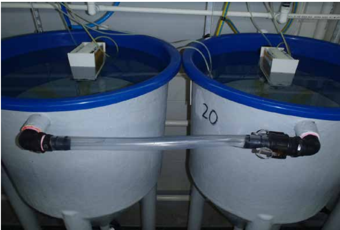
Figure 6. A pair of 270 Lt tanks connected during larval transfer
